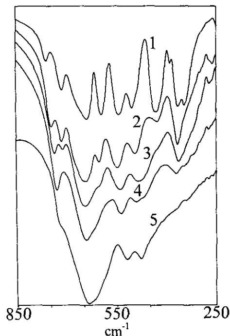
FIG. 3. Determination of the order–disorder transition P4_32 \rightarrow Fd3m by infrared spectroscopy in the \text{Li}_{0.5}(\text{FeCr})_x\text{Ga}_{2.5-2x}\text{O}_4 system. 1, x = 0 ; 2, x = 0.5 ; 3, x = 0.75 ; 4, x = 1 ; and 5, x = 1.25 .
